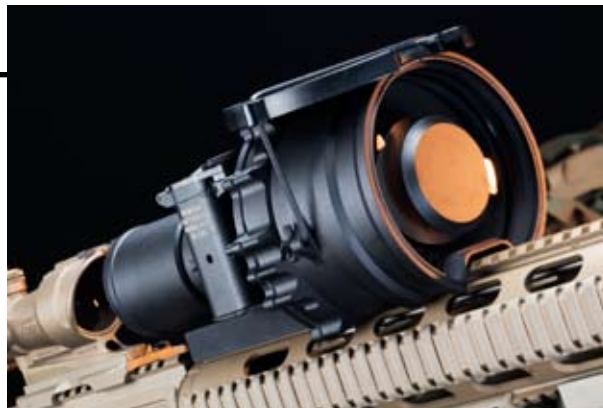
Generation 3+ AN/PVS-27 is USMC standard NVS and represents the highest light-gathering capability of any I 2 night vision device.
